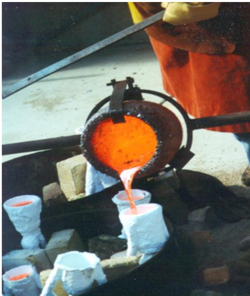
**This workshop** will introduce you to the “lost wax” investment casting process. You will be taken through all stages of lost wax ceramic shell casting, including spruing systems, ceramic shell application, bronze pouring, chasing & fettling, and some patination (metal finishing) techniques. The workshop will also introduce you to mould-making and possibly even sand-casting techniques.
